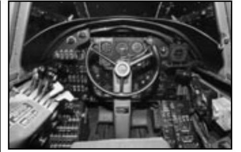
(above) The Douglas A-20 was controlled by one pilot with armaments and aviation control at the pilot's fingertips. A turret gunner flew in the A-20 as well.
