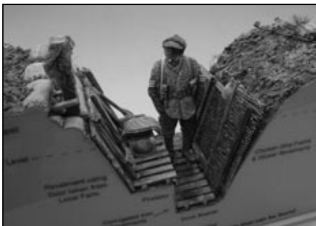
A museum diagram of a classic WWI trench, showing how the duck boards helped to keep soldiers' feet dry, helping them to avoid the wartime malady called "trench foot".
