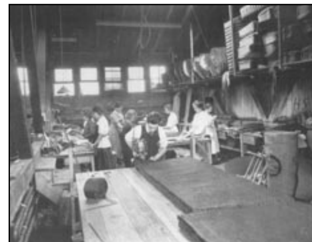
(above) Construction of an auto body at Superior involved much work by hand including sewing, and cutting upholstery. Most of the sewing was done by women.
