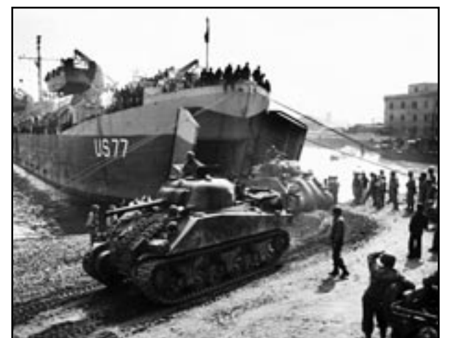
(above) The LCT, Landing Craft Tank, was a British invention. It made its battle premiere at Operation Husky and changed the nature of the amphibious landing from that day forward. Each transport ship could carry six medium tanks and was armed with rocket launchers and two 4.7" guns for self-protection. An incredible 1,435 were manufactured in American shipyards during WWII. They were used extensively at Normandy after the successes at the Battle of Sicily.
