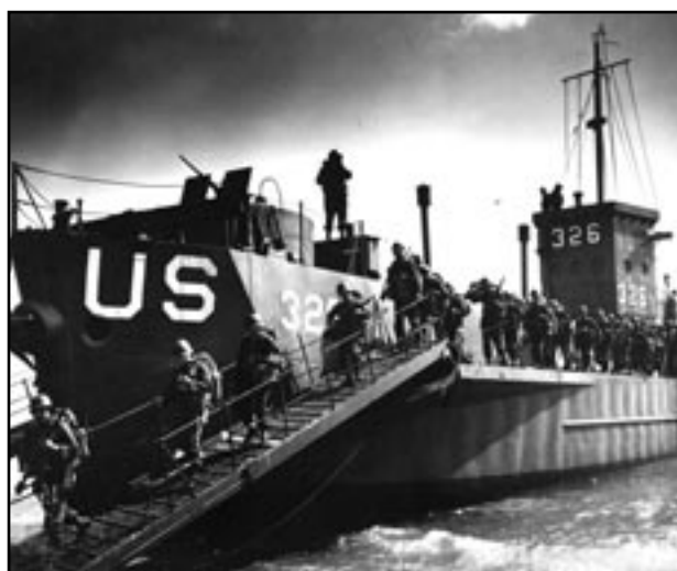
(above) The acronyms LCI, LCT and LCS are common in war stories which describe amphibious landings. We are extending our Cranford 86 "putting a face, to a name" slogan, to ID the 234 ton gorilla in the room. This LCI, or Landing Craft Infantry, is a much larger ship than the average reader might imagine. Each one, 158 feet in length, holds 200 fully geared soldiers. There were 923 LCI's manufactured during WWII.
