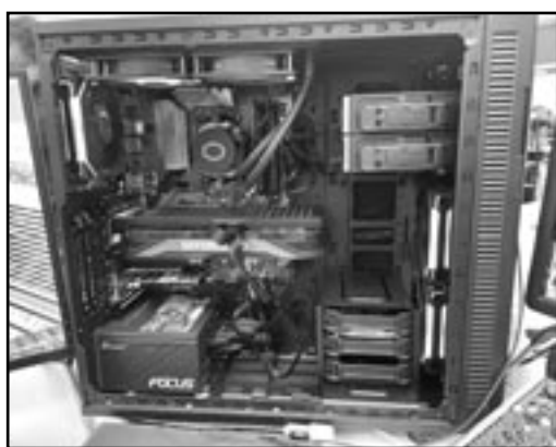
(above) The computer that students at McManus Middle School in Linden built piece by piece has a 32 MHz Ryzen 7 5800 Processor and 32 GB of RAM.
