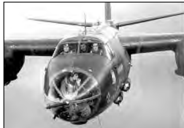
(above) The front view of the B-26, note the bombardier under the cockpit with full view of the terrain below.
